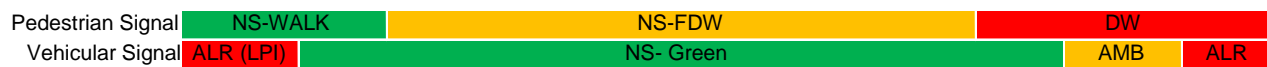
Figure 4 - Suggested trading of LPI Period at the End of the Walk Phase
